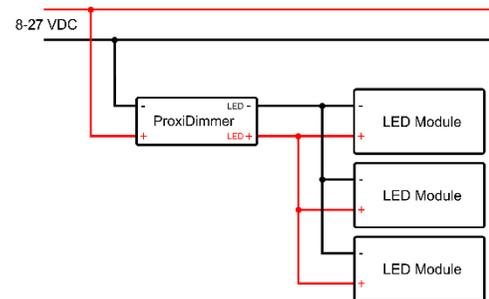
Above connection is an example and may be different from the actual. Wires between the power supply, controller and LED modules should be as short as possible. Connecting more than one controller to the same power supply is not recommended, it may cause interference, visible on LED light sources. Controllers adapted to such work are available on special request.
