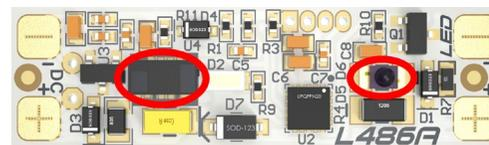
Components marked by red circuit are responsible for detecting objects, do not cover them with a material that doesn't pass infrared. ProxiDimmer sensor is working even with opal cover and automatically calibrating to it.
